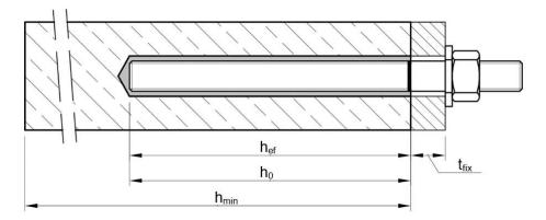
$t_{fix}$  = thickness of fixture
